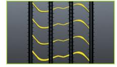
Shallow tread design reduces rolling resistance for better fuel efficiency.
